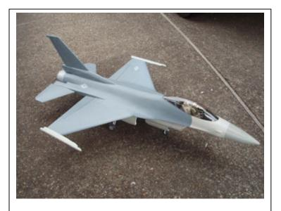
This is a Combat Models F-16N kit. It is all foam, weighs in around 8lbs, and has a YS 0.45FR pumped engine with a tuned pipe exhaust. I have only flown it a couple of times and still do not have the landings down yet, but it looks a lot like the real thing. Watching it go vertical on the first takeoff for a couple hundred feet was too cool.
