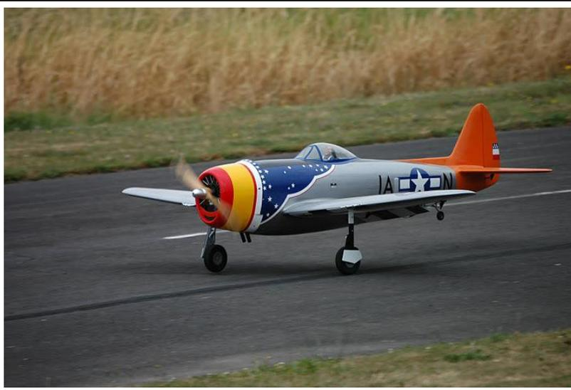
*John Vanloo's gaint scale P47 landing at OMAS 2011 air show. Power plant is OS GT55 gasoline engine, pitts exhaust. Flown by Darrin Miller.*
